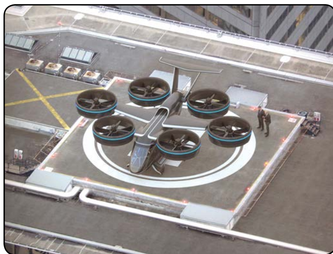
The Nexus is designed to fit into a 37 X 37-ft. size area typical of a light helicopter landing site and smaller than the 45-ft. box size allowed by Uber.
