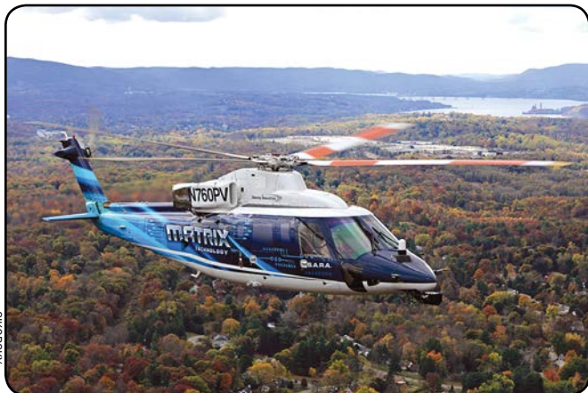
An S-76B modified to fly-by-wire control, SARA is Sikorsky's testbed for the Matrix autonomy system.
