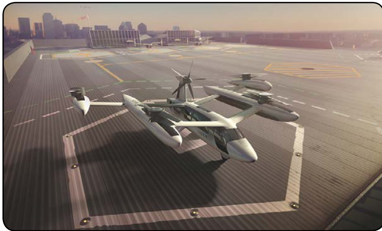
Uber's eCRM-003 is a distributed electric propulsion eVTOL concept with separate lift and cruise propulsion systems.
